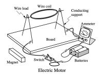
Motors coils should be ~4" in diameter with 4 windings of stiff wire. Each lead to the coil should be stripped of insulation for half of its circumference.
